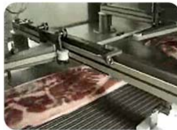
Click here for a video of the DSI 612 system, which sorts pork bellies by weight or thickness for optimized processing yields and reduced labor costs.
